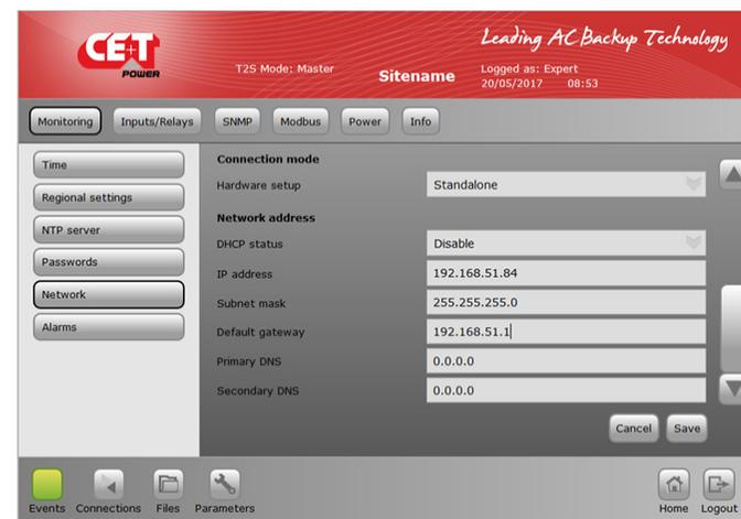
**Figure 4: Network parameters – to change**
